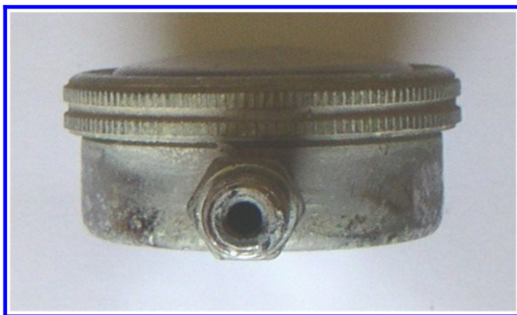
HP Pressure Gauge Inlet Clogged
