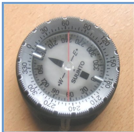
Suunto SK7 compass with graduated crown and details
