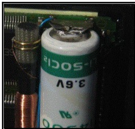
Welding the negative
