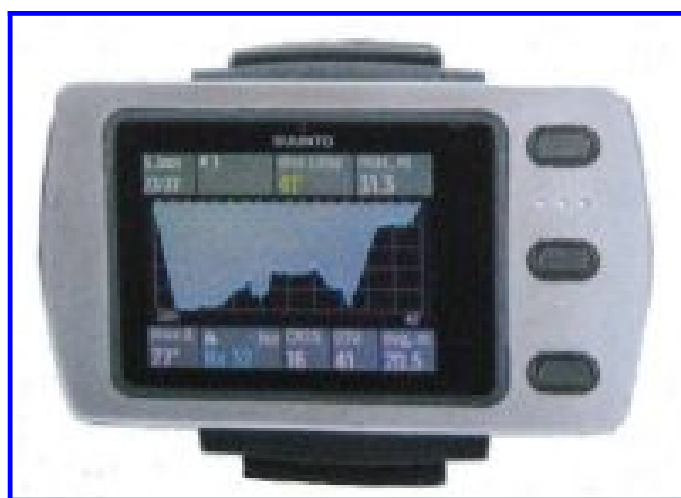
SUUNTO Eon Steel profile With organic light-emitting diodes (OLEDS)
